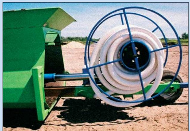
Perforated plastic aeration pipe is fed into the recyclable LDPE EcoPOD<sup>®</sup> composting bags and connected to timed aeration fans powered by a diesel generator.
