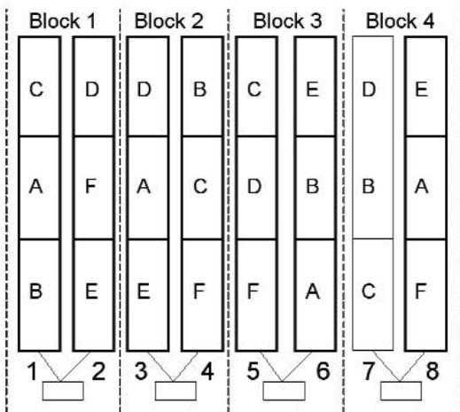
Six different mixtures of feedstock wastes were composted using EcoPOD<sup>®</sup> in-vessel composters. Each of the 8 EcoPOD<sup>®</sup>s was divided into 3 sections to allow replication of each mixture (x 4) in a randomised complete block experiment.
