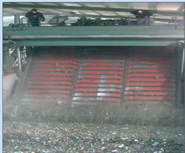
Fig. 2. Mechanical mixing of the wastes during the composting process.
